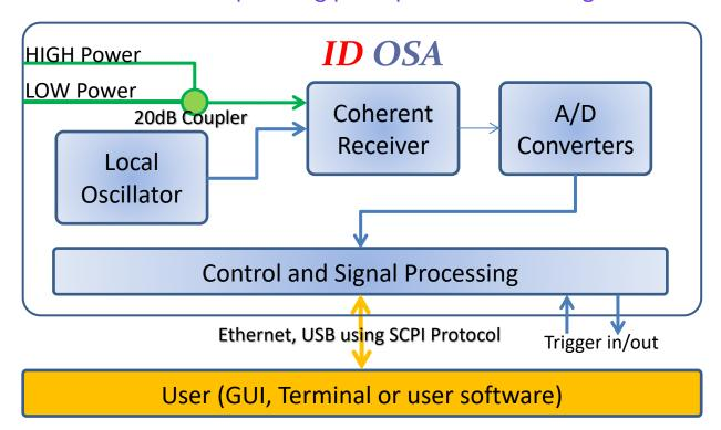
The ID OSA is an optical spectrum analyzer that provides two optical inputs measuring both higher power signal spectra and signals requiring a high sensitivity by means of an integrated coupler across the C Band. The unit automatically corrects the reported power once the user has selected the input currently in use.
