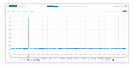
Use the slider shown below the graph to zoom into areas of the measured data. The data outside of the zoomed area is still measured and depicted in the slider. The selected area can be moved by dragging the selected area with the cursor. Alternatively, it is possible to zoom in via marking the area of interest using the cursor in the main graph.
