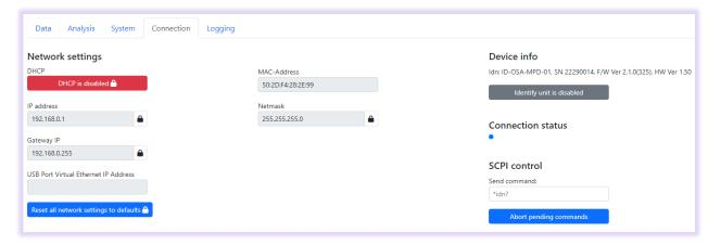
This tab is used to retrieve or set information on the remote-control interfaces of the unit, device info and information about current firmware and identification of the unit. Hover the cursor over the fields to access a detailed description of them.
