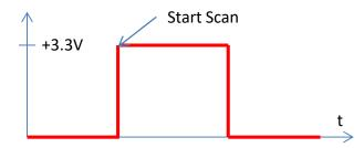
Trigger OUT provides an output signal indicating periods at which the unit acquires the optical spectrum. The polarity can be reversed via Remote control or GUI.
