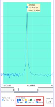
Use the checkboxes located in the lower part to make the channel mask of detected peaks visible and show analysis results.
