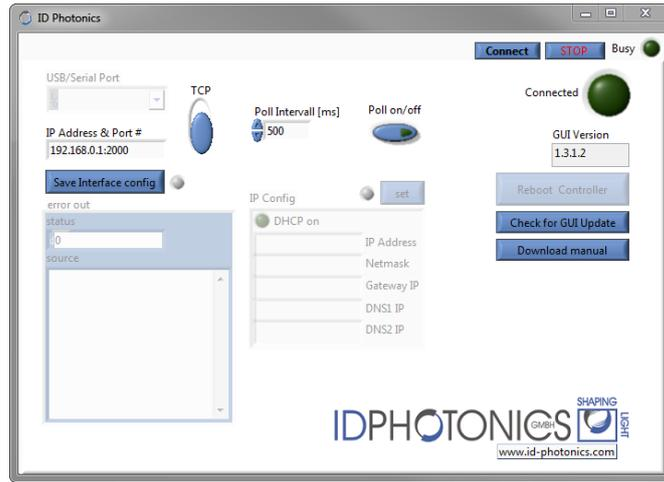
Once the GUI has connected to the instrument, the GUI will display the Interface configuration and the previously disabled Tabs become available. The “Connected” indicator will be solid green. The “Busy” indicator will flash each time the GUI’s readings are updated. The interval time can be changed by setting the “Poll interval” parameter.
